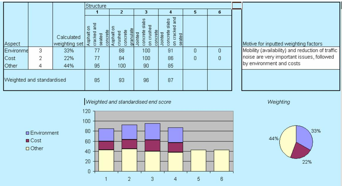
Figure 4 MCA results for 4 pavement options after weighting
